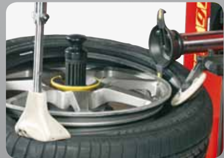
• Con premitallone (accessorio a richiesta) • With bead pressing clamp (optional accessory)
