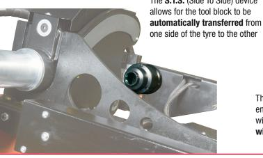
The **S.T.S.** (Side To Side) device allows for the tool block to be **automatically transferred** from one side of the tyre to the other
