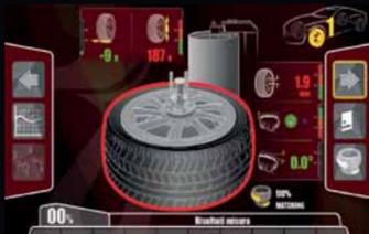
**iPos:** a special program for positioning the four wheels in the best possible way to guarantee the driver's comfort and safety.
